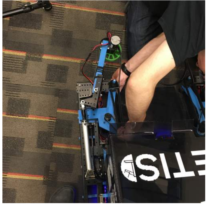
Fig. 6. A view of the actuated intake from the top
