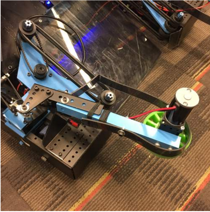
Fig. 4. A look at the elastic joint– the blue bar pivots around the bolt attaching it to the black part
