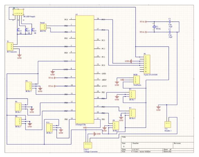
Figure 7. PCB Schematic Diagram
