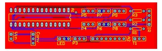
hardware design. We printed a single circuit board to verify the connections before producing the *Figure 5. Prototype PCB design sketch*
