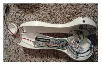
Figure 5. Exposed PCB in the device case
